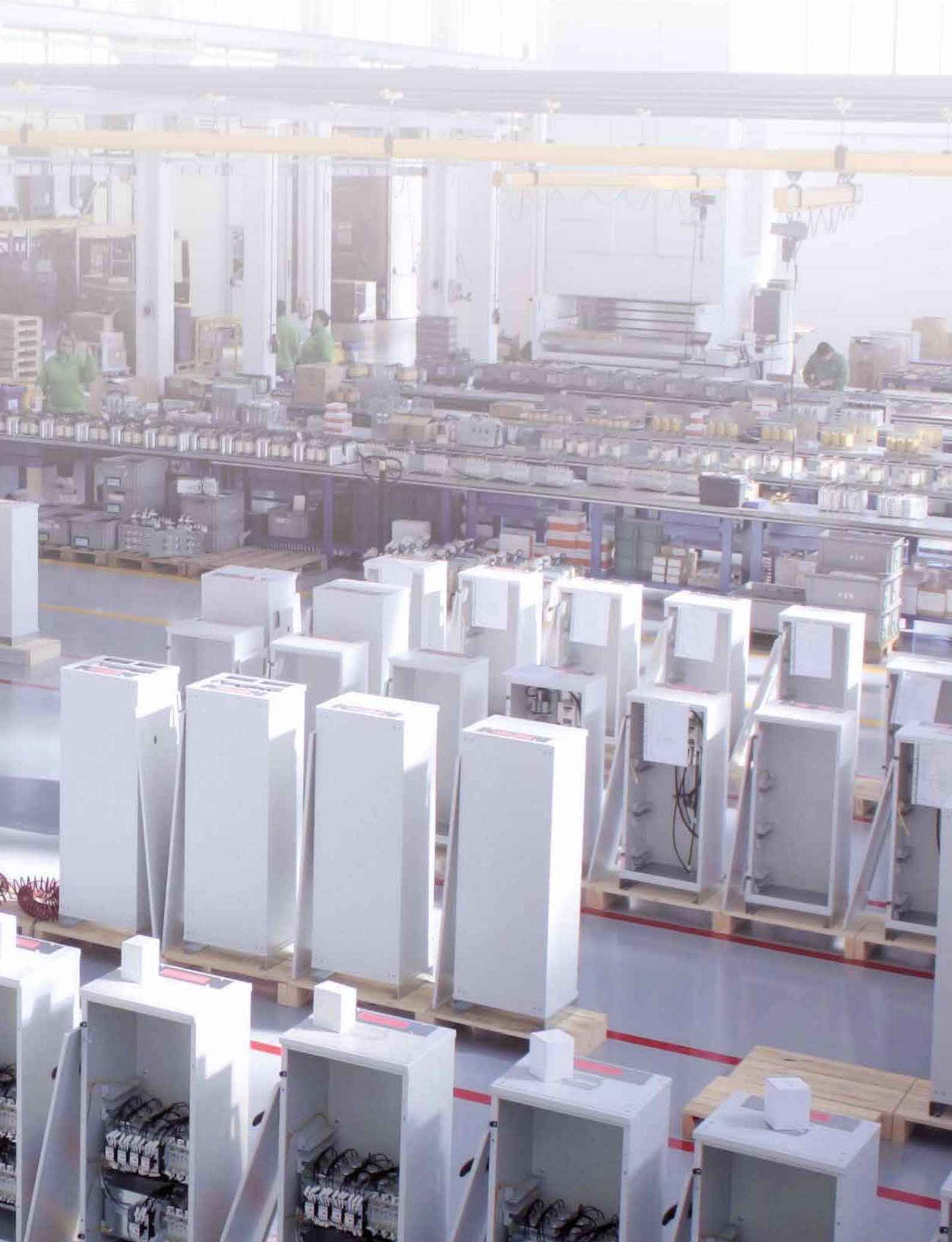
PRODUCTION OF POWER FACTOR CORRECTION BOARDS AT THE PLANT IN CAVENAGO DI BRIANZA (ITALY)
